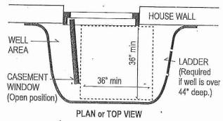
Note: Centering a window well at the window might not give you the required minimum 36 inches. Measure carefully!
