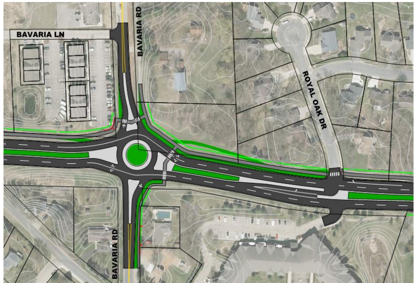
Figure 19. Proposed Roundabout at Bavaria Road and Three-Quarter access at Roval Oak Drive.
