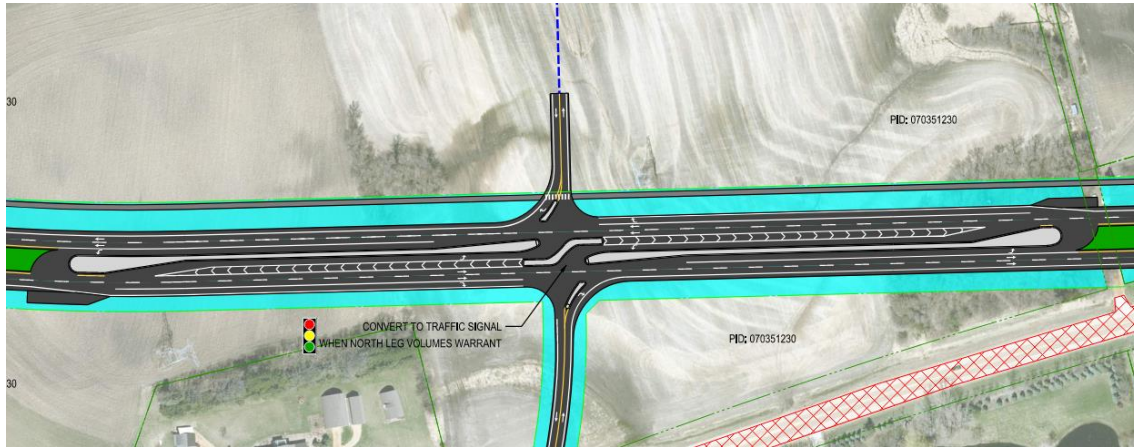
Figure 36. Highway 43 East at Highway 10 Reduced Conflict Intersection.
