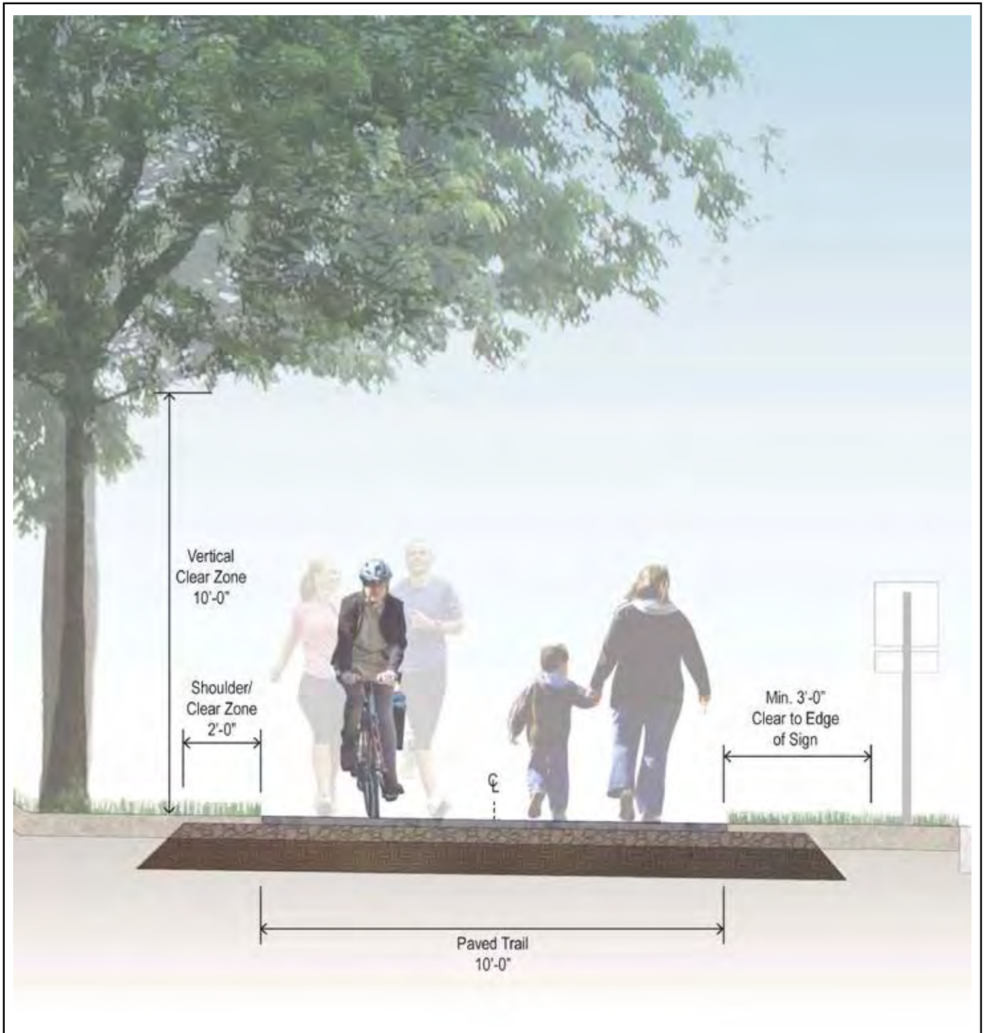
Typical Trail Cross-Section Figure 4
