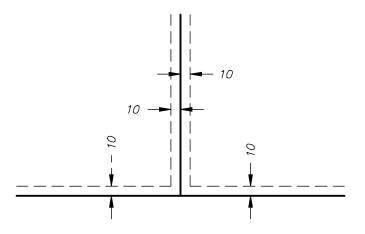
Drainage and Utility Easements being 10 feet in width and adjoining right of way lines, and being 10 feet in width and adjoining lot lines, unless otherwise indicated.
