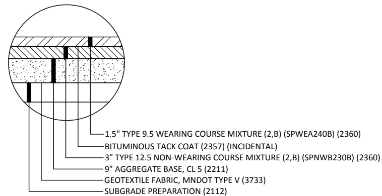
BITUMINOUS TYPICAL SECTION
